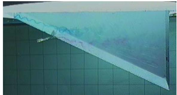
12a blowing under vortex core
