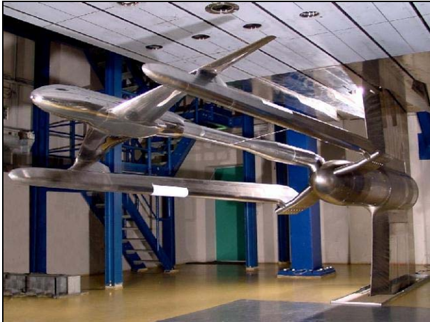
Figure 18 Model installed on the twin sting rig
