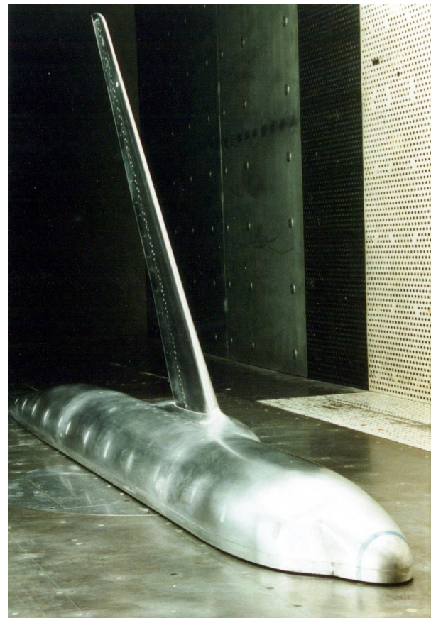
Figure 11. Semi-span model installed in TWT
