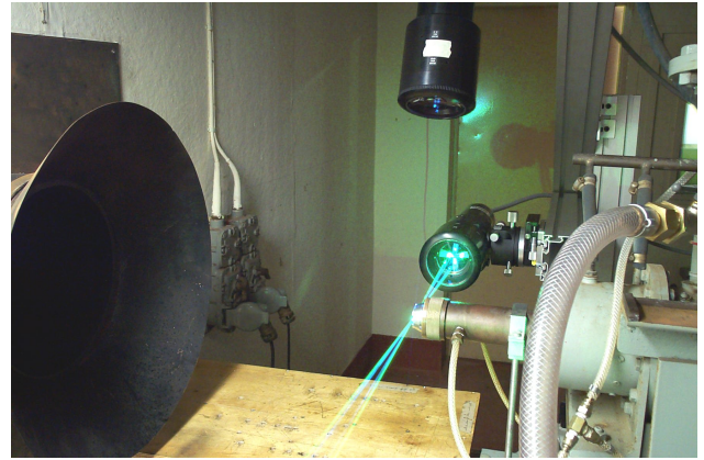
Fig. 3 LDV measurements in the nozzle test cell.
