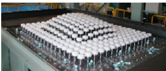
Fig. 20 Multi support core molding jig
