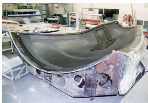
Fig. 21 sandwich panel molding jig
