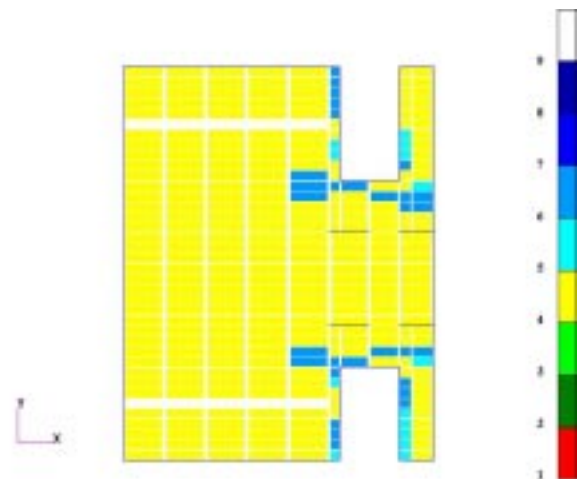
Fig. 8. FML panel failure modes.
