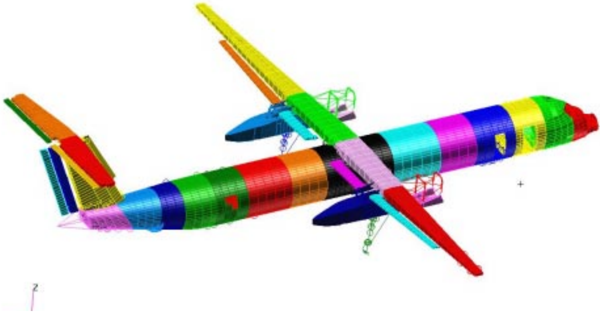
Fig. 1. FEM model of Dash8-Q400 aircraft illustrating substructures.
