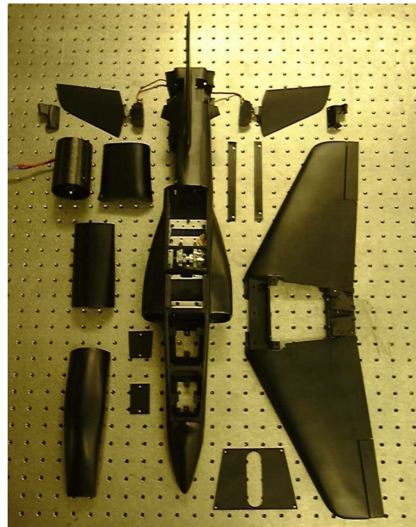
Figure 5: Disassembled Hawk model, showing various components
