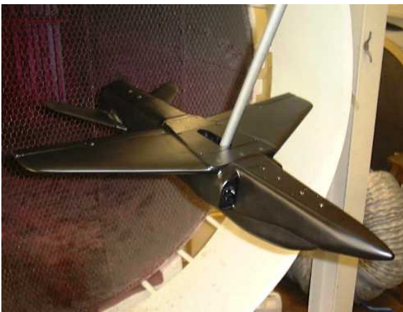
Figure 3: Pendulum rig layout in open-jet tunnel.
