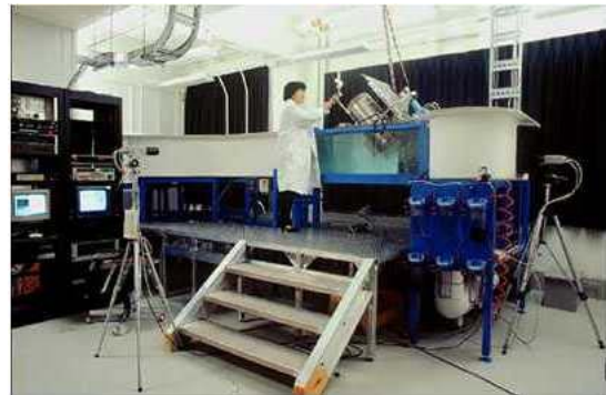
Fig.1 General arrangement of experimental equipment in IAR water tunnel
