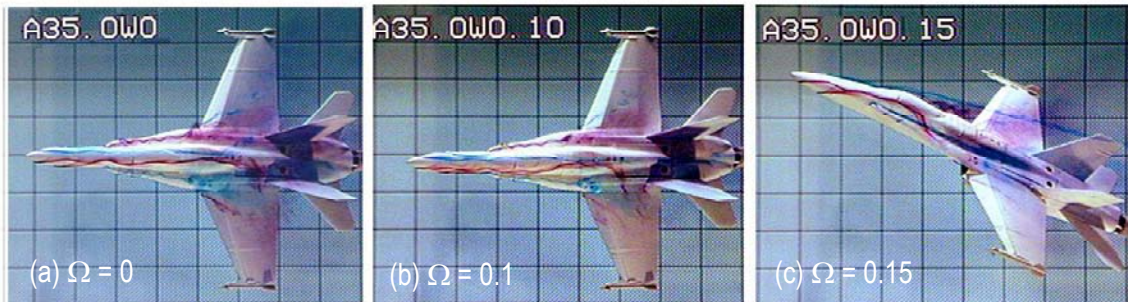
Fig. 8 Rotary flow pattern at \alpha = 35^\circ
