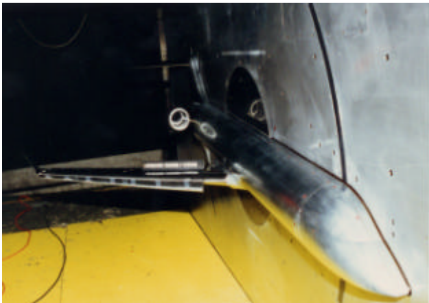
Figure 13: 7 percent scale half-model of the CRJ-700 installed in the IAR 5-ft high Reynolds number wind tunnel
