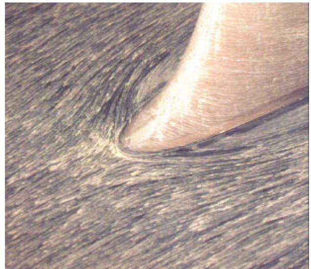
Figure 7: Effect of the fairing on the flow near the wing-plate junction (The picture on the right shows the small fairing)
