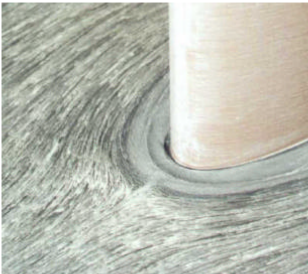
Figure 7: Effect of the fairing on the flow near the wing-plate junction (The picture on the right shows the small fairing)
