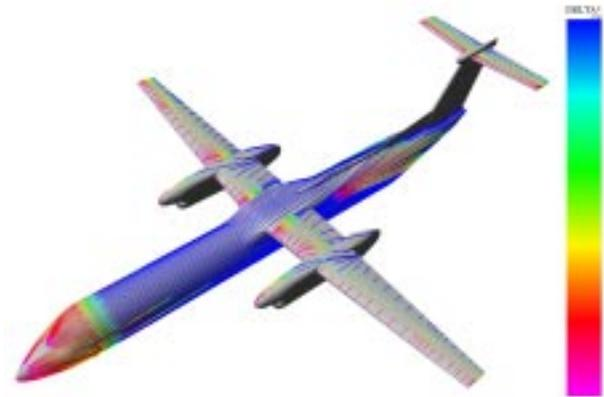
**Figure 4 Surface displacement thickness**
