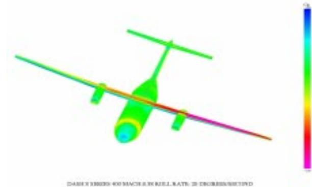
**Figure 11 DASH 8 400 pressure distribution at 20 deg/sec roll rate M:0.58**
