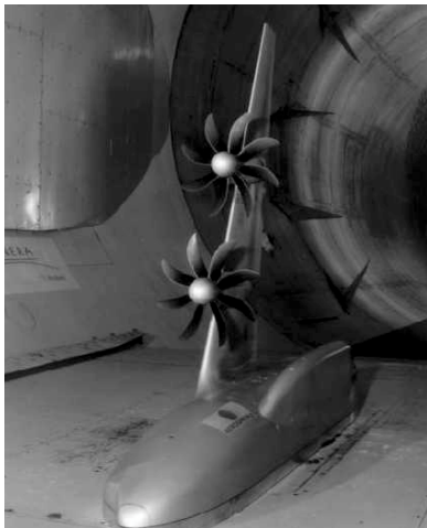
Figure 6: The half-model of the Generic Transport Aircraft in the SIMA wind tunnel.
