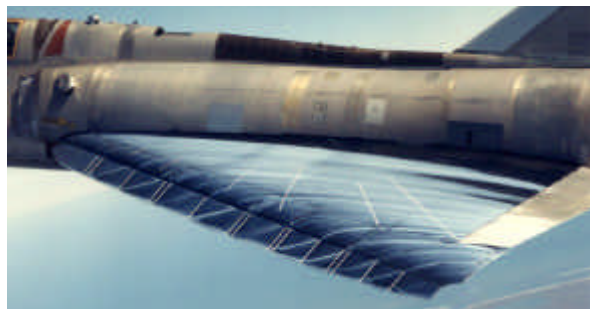
Fig. 16- In-flight vortex flap flow-visualization result. \alpha=10^\circ , \delta_f = 40^\circ . Brandon et. al. [24]
