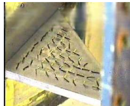
g) The tuft visualization result, \alpha=10^\circ [12]
