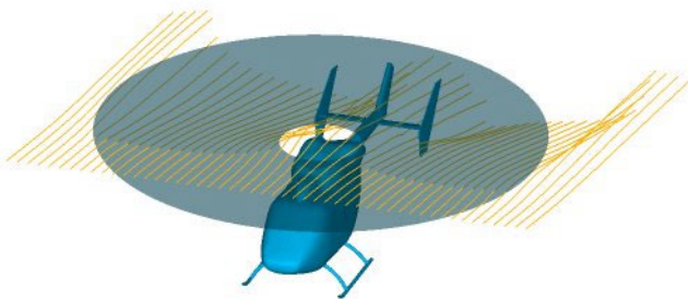
Fig. 17. Visualization of streamlines from linear seeds.
