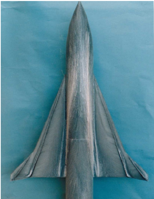
Figure 6-(a) Top view with lateral blowing ( \alpha=10^\circ , M_\infty=0.3 at Case1)
