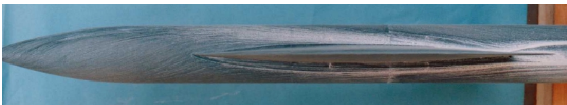
Figure 6-(d) Side view without blowing ( \alpha=10^\circ , M_\infty=0.3 at Case1)
