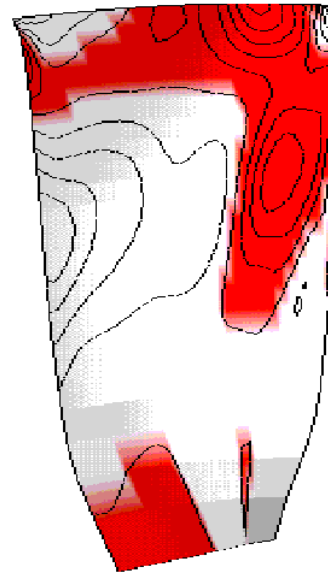
Figure 12 : 3D Euler unsteady supersonic flutter analysis : Mean power distribution
