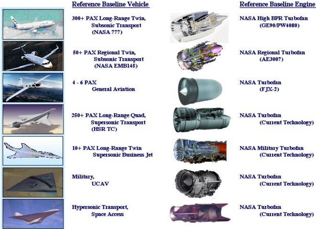
Figure 4. Reference vehicles and propulsion systems used to assess UEET technology benefits .
