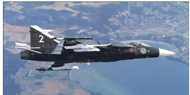
Figure 12. Test a/c 39-2 with anti stall chute.
