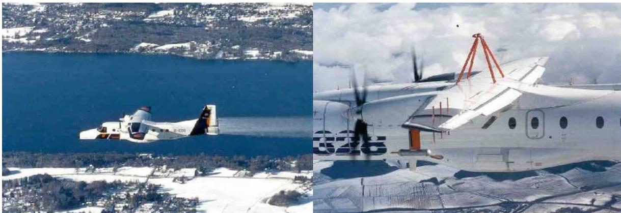
Figure 1: Dornier ice tanker (DIT) and following test aircraft (TAC) equipped with OAP-1D sensing probe, ice accretion cylinders and video camera
