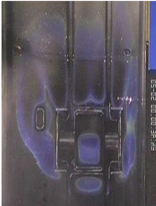
Figure 9. Video camera view of intercase model showing liquid crystal colour change.
