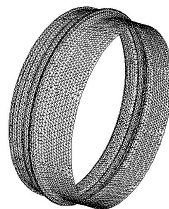
Figure 6: Annular surface mesh obtained by rotating the surface mesh above
