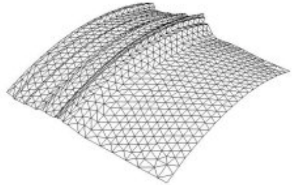
Figure 5: Surface mesh on a 45 degree section of a body of revolution (Trent 500 zone 3)
