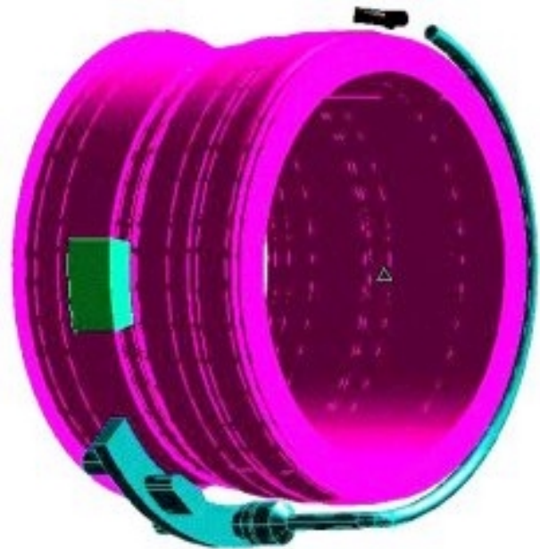
Figure 3: Starboard view of inner casing of filtered geometry – Trent 800 zone 1
