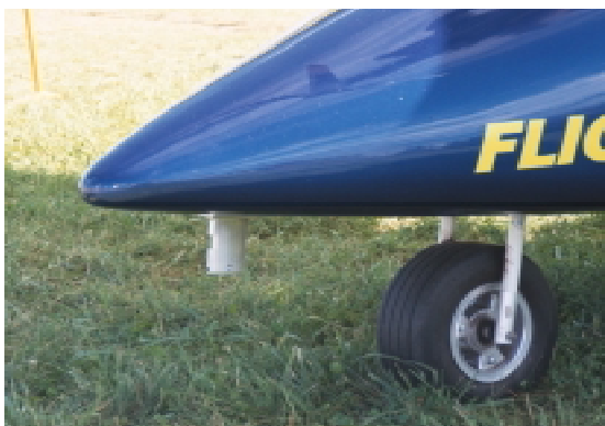
Figure 13. EPIREPS sensor mounted under nose of light aircraft
