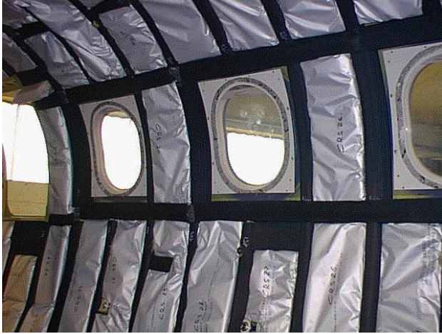
fig. 1: above floor PC12 insulation concept.
