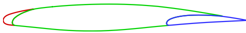
Fig. 1 Cruise flight reference configuration (based on the 3 element high-lift configuration BAC 3/11/RES/30/21 [7])
