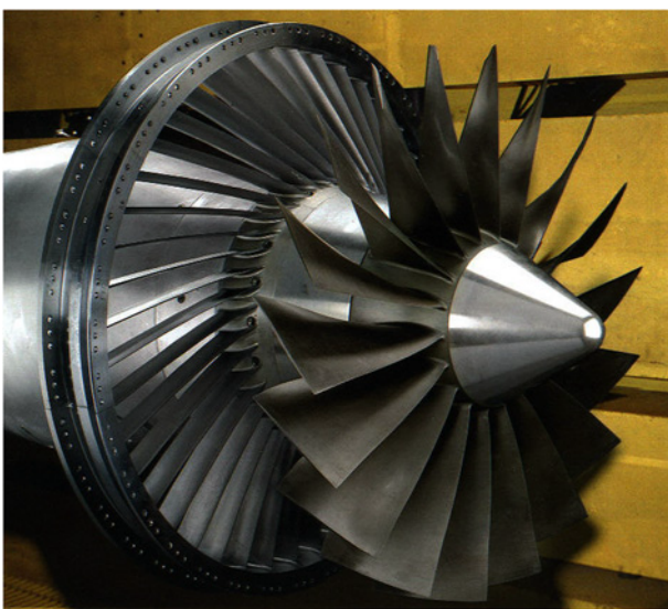
Figure 6. Model-scale swept and leaned stator used in wind tunnel acoustic tests shown with fan and without nacelle
