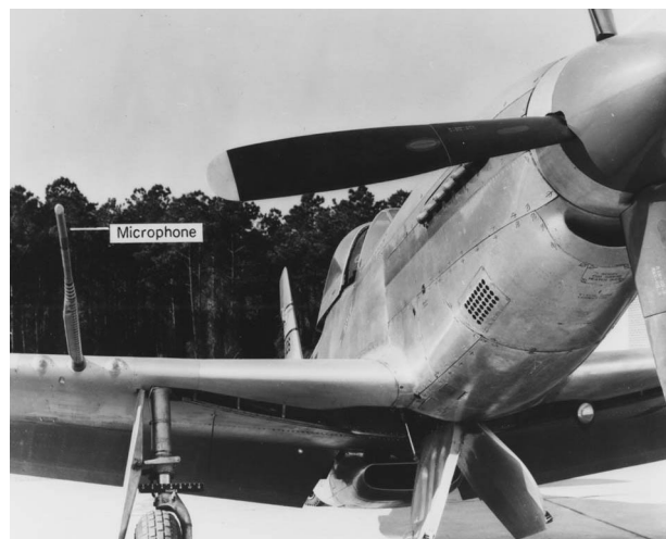
Figure 1. Early NACA propeller noise test on a P-51 fighter airplane.
