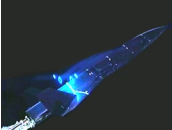
Figure 8. Wind tunnel visualization of flow around the MTVI configuration showing chine vortex burst.
