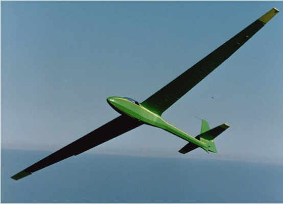
Fig. 1: EA-9 “Optimist” glider in flight, (single-seat, span 15.7m, maximum take-off mass 335kg), courtesy J. Edgley.
