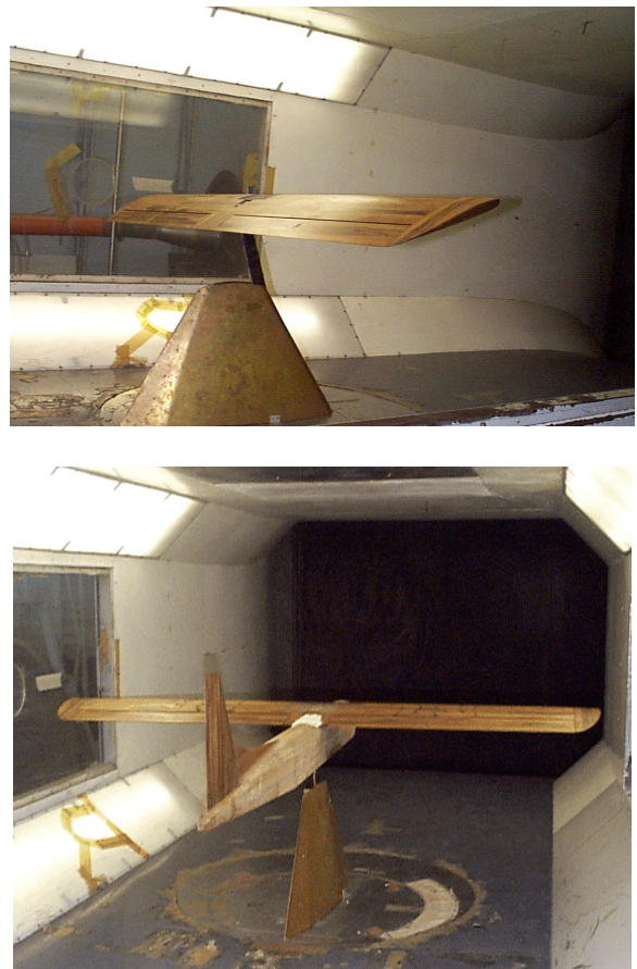
fig. 4 – Wing and wing-body configuration in the 2x1.4 m test section wind tunnel
