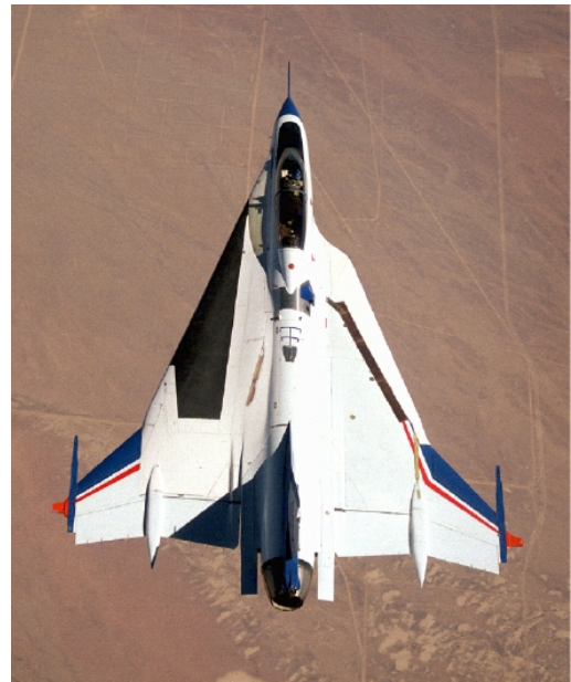
Figure 4. Laminar flow control system demonstrated on a F16-XL at Mach 2.0.
