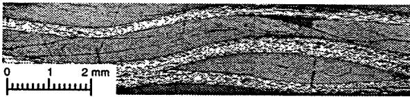
FIGURE 5 - Photomicrograph of a braided composite showing crimp of the axial fibre tows
