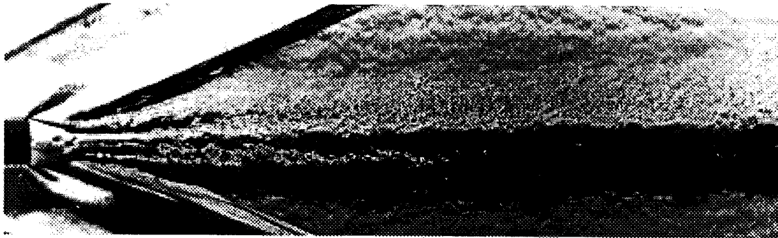
a) mixing layer with 1 slot jet on
