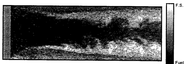
Figure 8. Quantitative image of freestream and fuel mole fraction for the plane-base injector. The injector's position is shown by the grey mask at the left of the image. The scale to the right indicates the amount of freestream gas.
