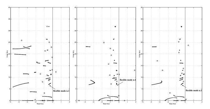
**Fig. 3** Root loci at  $m_1$  for the initial  $\mathcal{H}_2$  controller (on the left), the intermediate (in the middle) and the final modal dynamic controller  $K_0(s)$  (on the right)
