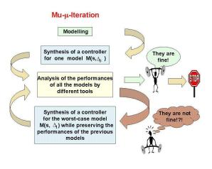
**Fig. 2** The multi–model (Mu- $\mu$ )–Iteration
