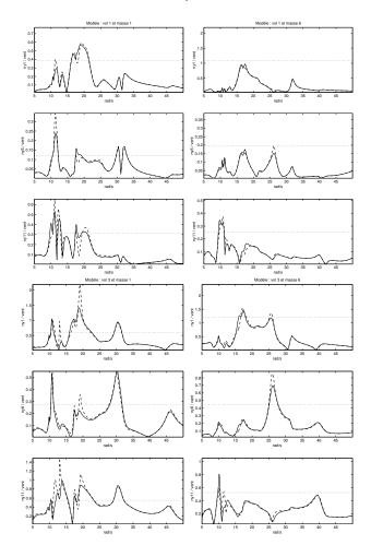
**Fig. 5** Frequency domain responses of lateral acceleration  $n_{y,i}$  of the initial  $\mathcal{H}_2$  controller (dashed line) and the dynamic modal self–scheduled controller  $K_{sched}(s, \delta V)$  (solid line) for the two models  $m_1$  and  $m_6$  at speeds  $V_1$  and  $V_3$
