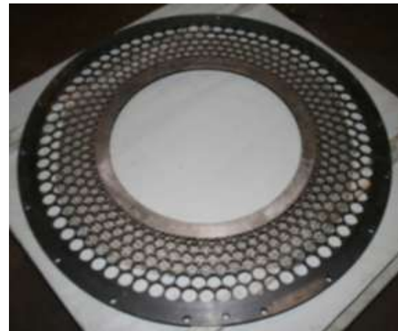
Distortion screen unit for simulation designed radial flow non-uniformity at the stage inlet
