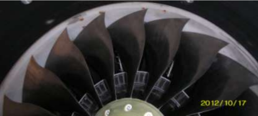
C180-2 fan model (variable swept blade and forward swept in tip section blade)
