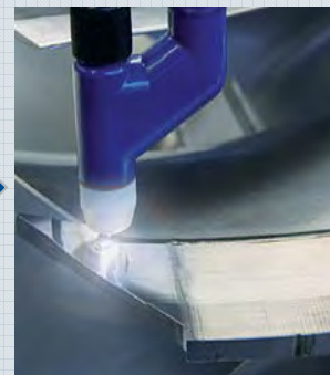
Patching of compressor Blisks by Plasma Welding
