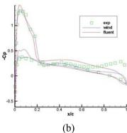
Fig. 11 Pressure coefficients at section y/b= (a) 0.2 (b) 0.99
