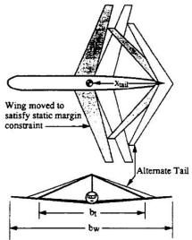
Fig. 2 Typical joined wing aircraft with two alternate tails [1]
