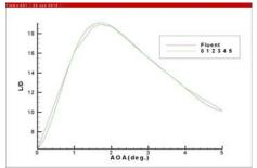
Fig. 12 L/D comparison between Kriging prediction of AOA=0°, 1°, 2°, 3°, 4°, 5° and FLUENT solver for BWB with no engine
