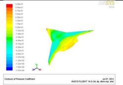
Fig. 13 Pressure contour for BWB at 0.85 Mach and 2.09 degree with engine position of 2.97m.
