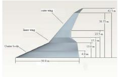
Fig. 5 Blended-Wing-Body geometry model [22]
