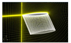
Fig. 10 Near structure mesh of the M6 wing
