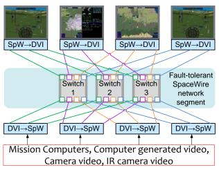
Fig. 5 Fault tolerant fly-by-wire systems; 2 failures tolerant cockpit interconnection
