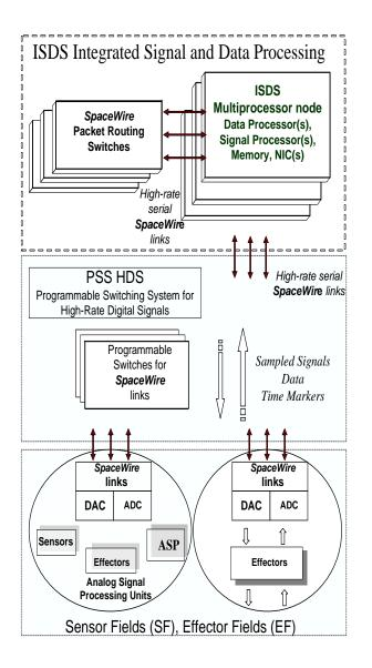
Fig. 1. Distributed Integrated Modular Spacecraft Avionics Architecture
