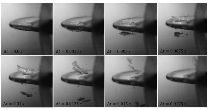
Figure 8. Deicing sequence of a sample glaze icing condition shot with a high speed camera.
