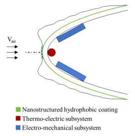
Figure 1. Working principle of the hybrid ice protection system.
