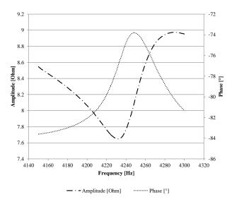
Figure 6. Reactance of the hybrid ice protection system.
