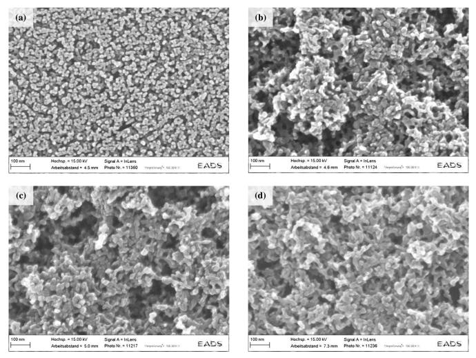
Figure 3. Top-view SEM images of the anodized samples at (a) 18 V/20  $^{\circ}$ C, (b) 18 V/26  $^{\circ}$ C, (c) 18 V/30  $^{\circ}$ C, and (d) 22 V/26  $^{\circ}$ C
