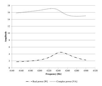
Figure 7. Power consumption of the hybrid ice protection system.
