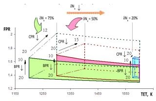
Fig. 4. Cruise design parameter ranges of HGTE-1 for kerosene (R=1200 kgf, H=11 km, M=0,78)
