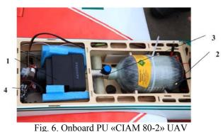
1 - Aeropak PEM FC battery, 2 - fuel tank, 3 - gas pressure regulator, 4 - control system
