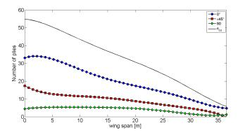
**Fig. 6** Number of plies per each orientation and total number of plies along wing span for panel 4
