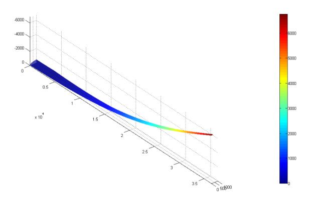
**Fig. 8** Wing box deflection at iteration 20
