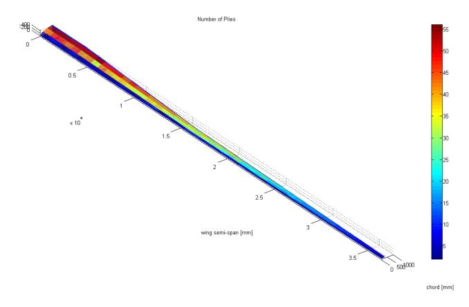
Fig. 7 Number of plies at iteration 20
