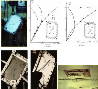
Fig. 3 Undamaged and Damaged buckling results of panels under shear loads
