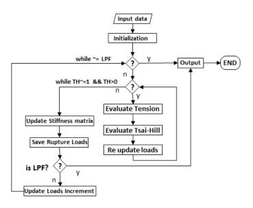
Fig. 2 Progressive Ply Failure Analysis block diagram
