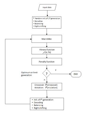
Fig. 4 Block diagram of the developed GA
