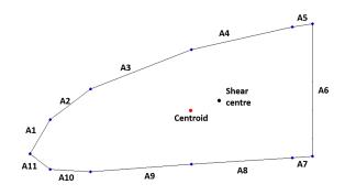
**Fig. 5** Wing box cross section discretization, section A (root section)
