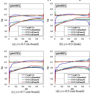
Fig 12. Cp distribution on the wing surface.
