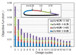
Fig 15. Breakdown history of the objective function on the upper surface (Case B).
