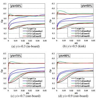
Fig 13. Enclosed *Cp* distribution around the L.E.
