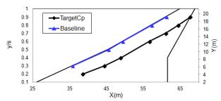
Fig 5. Estimated boundary layer transition on-set (*N*=14) of the high-*Re* consition (LSST).
