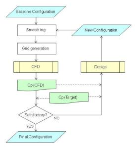
Fig 3. Design process of the NLF wing.
