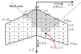
Fig 7. Coordinates and panels for formulation of the inverse problem of wing design [8,9,10].
