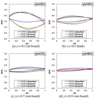
Fig 14. Designed airfoils.
