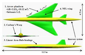
Fig 1. NEXST-1 configuration [1,2].
