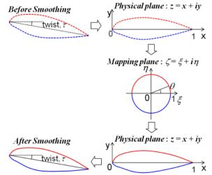
Fig 6. Smoothing image by conformal mapping [14,15].
