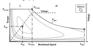
Fig. 1: Design chart of an electric machine showing important design points.
