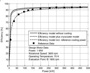
Fig. 4: Comparison of efficiency model of a HTS motor (only rotor) with reference data from [19]
