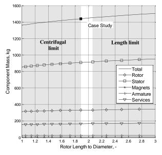
Fig. 6: Trade study of different rotor length to diameter variation at 22 MW and 11000 rpm
