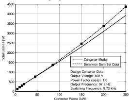
Fig. 5: Comparison of converter model with manufacturer data [26]
