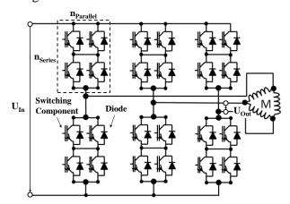
Fig. 2: Voltage Source Inverter for control of a 3-phase electric motor
