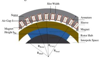
Fig. 3: Principle geometric design of the electric motor based on [15]
