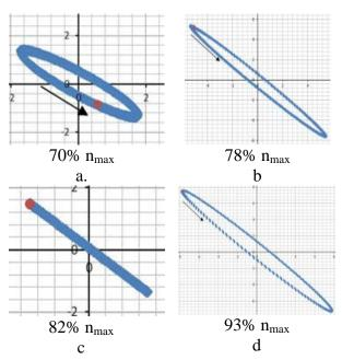
Fig. 8. Example of fan supports vibration displacement trajectory alterations during speed up (c – moment of degeneracy to line)
