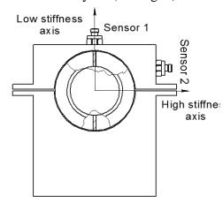
Fig. 3. The basic sensors mounting scheme
