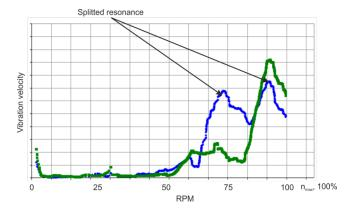
Fig. 7. Example of amplitude-frequency diagram. Green – sensor placed in vertical plane pf engine, blue – sensor placed at 20 degree to vertical plane (blue) of engine
