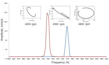
Fig. 4. The basic sensors mounting scheme investigation results (accelerometers signal FFT, red – sensor measuring horizontal vibration component, blue – sensor measuring vertical vibration component)
