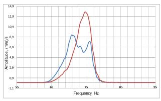
Fig. 6. The alternative sensors mounting scheme investigation results (accelerometers signal FFT, red – sensor measuring horizontal vibration component, blue – sensor measuring vertical vibration component)
