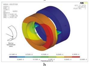
Fig. 2. Deformations of bush with two-axis stiffness anisotropy (a – deformation toward weak direction, b – deformation toward strong direction)
