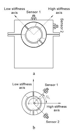
Fig. 5. The alternative sensors mounting scheme
