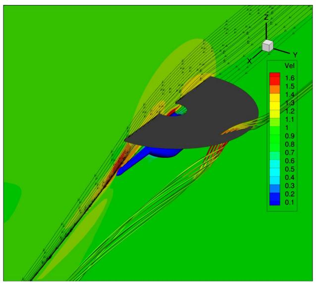
Fig. 1. Reproducible phenomenon: downwash and tip vortices
