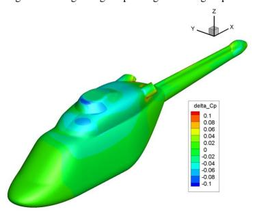
Fig. 6. Difference of pressure coefficient for uniform and non-uniform disc actuator load distribution
