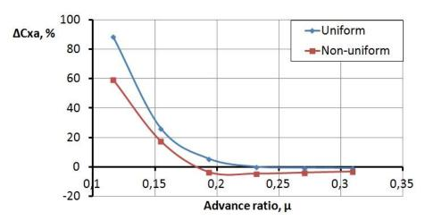
Fig. 5. The drag change depending on the flight speed
