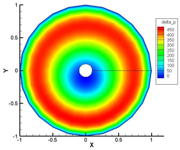
Fig. 3. Nonuniform distribution of the additional pressure (Pa) on the actuator disc
