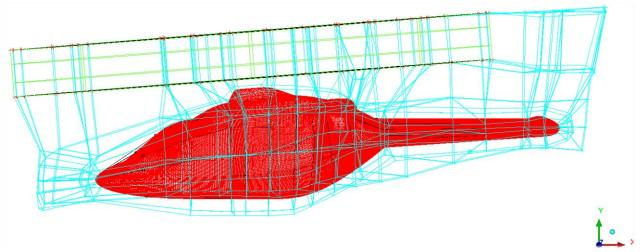
Fig.4. Bloking near the fuselage
