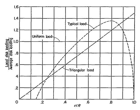
Fig. 2. Typical load distribution on the blade (NACA TR 1319)
