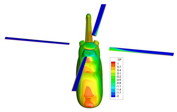
Fig.8. Pressure distribution on the helicopter: collective pitch  $\theta$ =8°; cycle pitch  $\theta_C$ =2°,  $\theta_S$ =-2°; advance ratio  $\mu$ =0.15; freestream Mach number M=0.1
