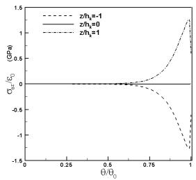
Fig. 3. Distribution of interlaminar shear stress in the interfaces of [90°/0]<sub>s</sub> panel, (R/h=30, 2b/h=8)
