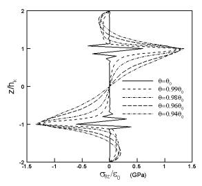
Fig. 5. Distribution of interlaminar shear stress  $\sigma_{\theta z}$  through the thickness in [90°/0]<sub>s</sub> panel under uniform axial strain  $\epsilon_0$ , (R/h=30, 2b/h=8)
