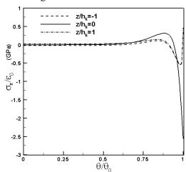
Fig. 2. Distribution of interlaminar normal stress in the interfaces of [90°/0]<sub>s</sub> panel, (R/h=30, 2b/h=8)
