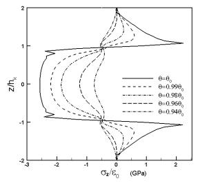
Fig. 4. Distribution of interlaminar normal stress  $\sigma_z$  through the thickness in [90°/0]<sub>s</sub> panel under uniform axial strain  $\epsilon_0$ , (R/h=30, 2b/h=8)
