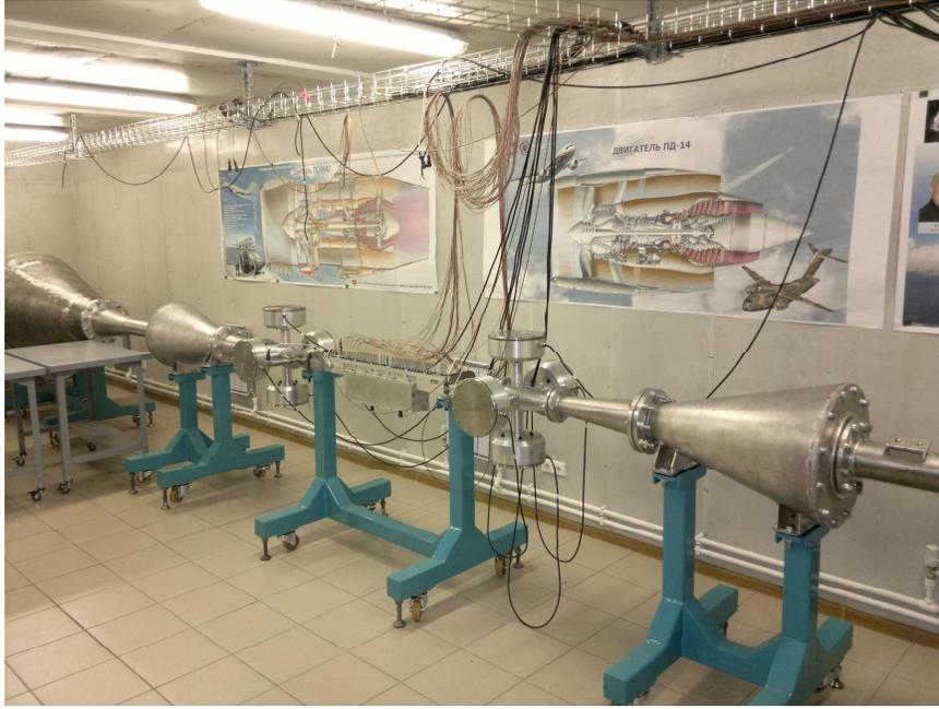
Fig. 1. Duct with flow facility in the PNRPU Acoustic Research Center
