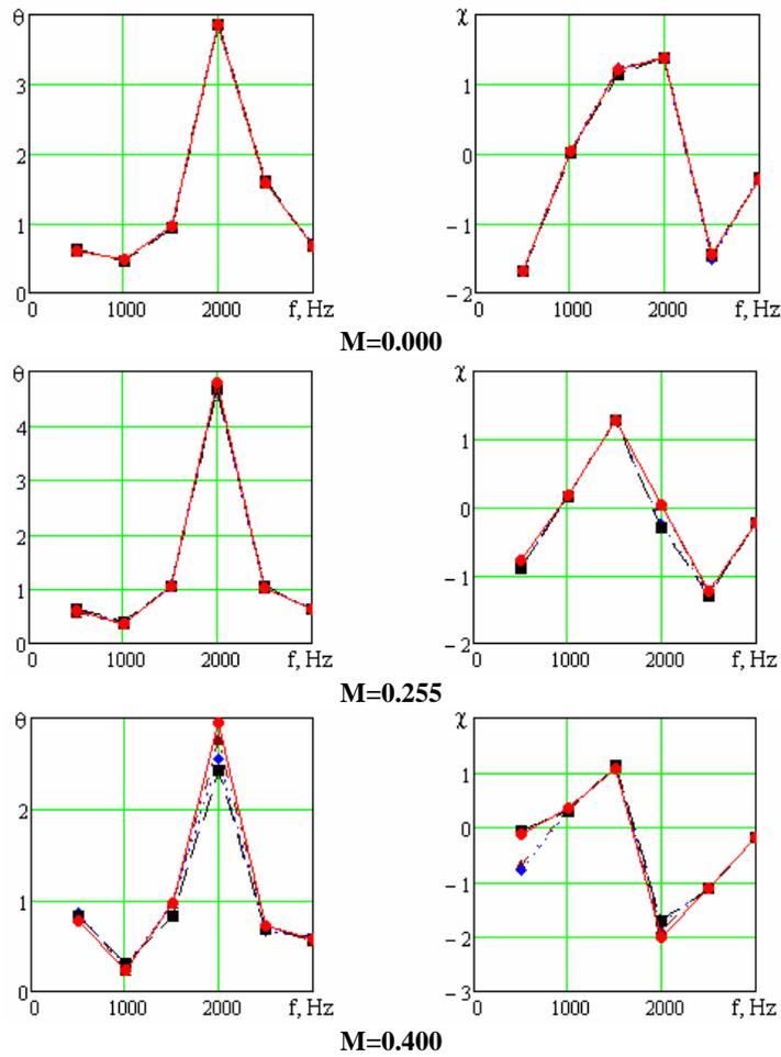
Fig. 8. Liner impedance at different number of microphones
