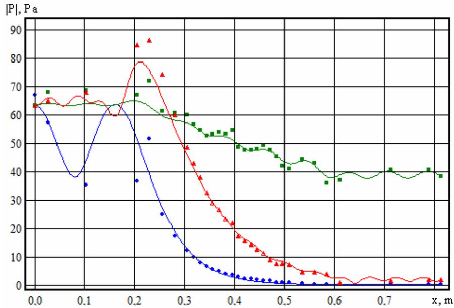
Fig. 5.1. Acoustic pressures on microphones ( $M = 0.225$ , 31 microphones)
