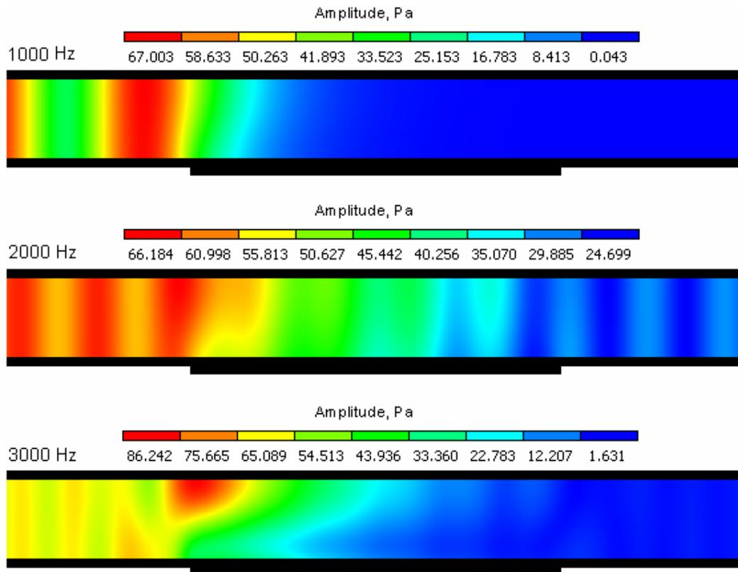
Fig. 4.2. Acoustic pressures in the duct with flow ( $M = 0.000$ , 31 microphones).
