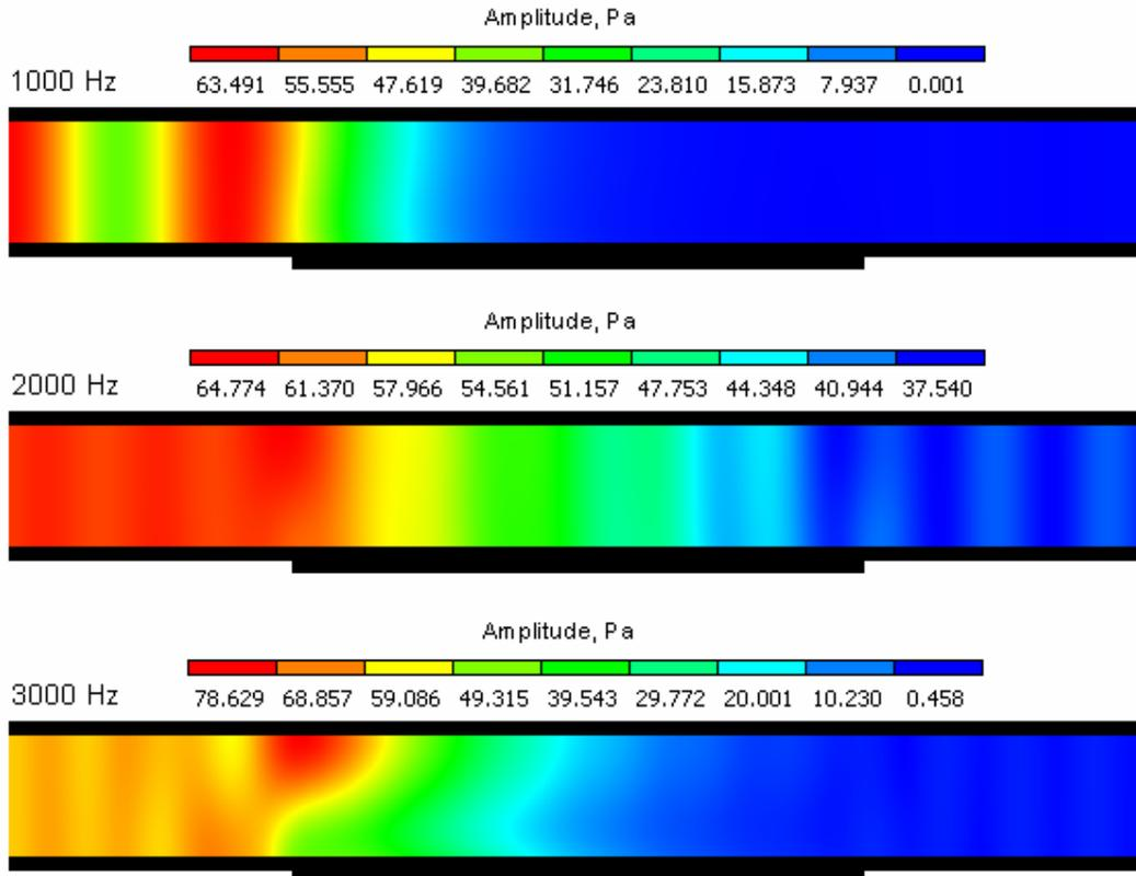
Fig. 5.2. Acoustic pressures in the duct with flow
