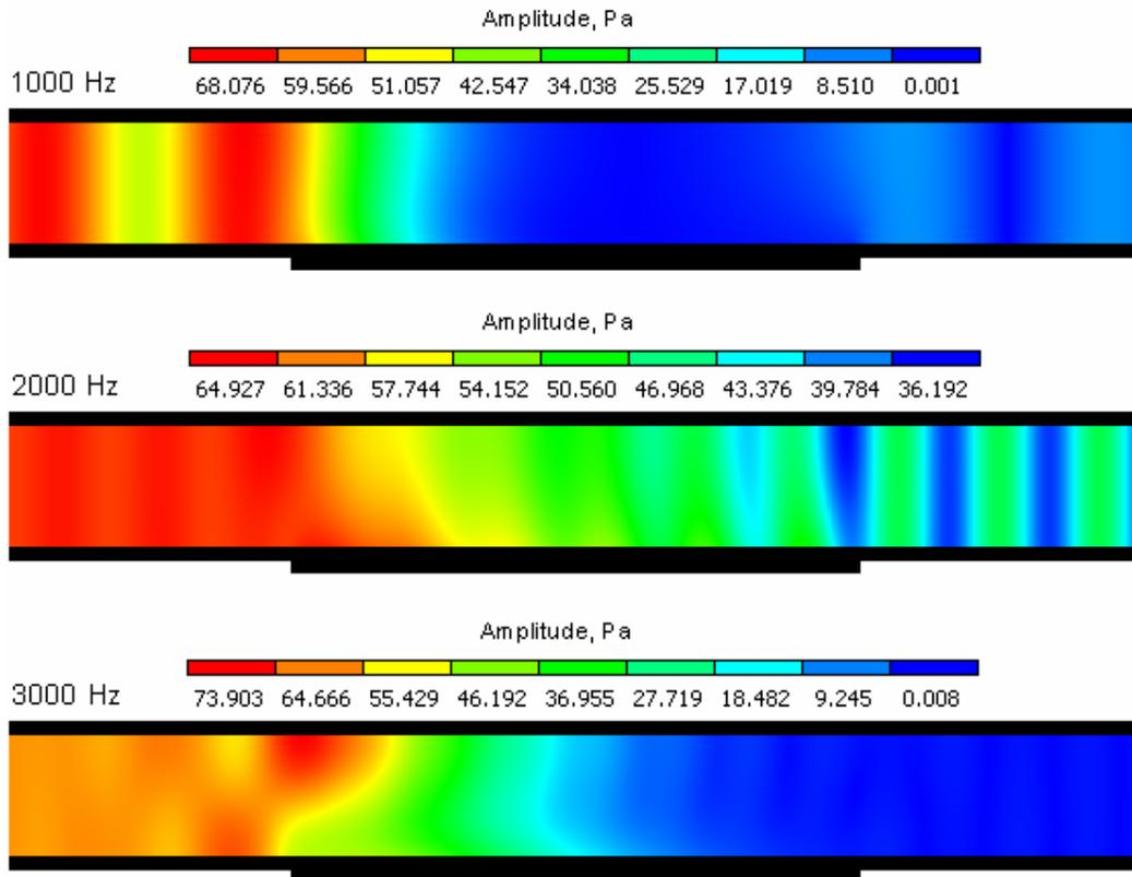
Fig. 6.2. Acoustic pressures in the duct with flow
