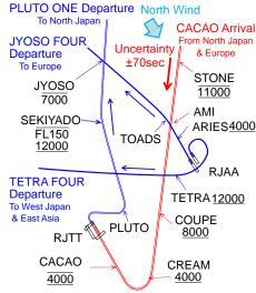
Fig. 7 Schematic of STAR and SID of RJTT and RJAA at north wind operation
