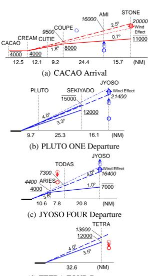
(d) TETRA FOUR Departure Fig. 8 Increase in Altitude with applying CDO and CCO and the change of altitude caused by north wind effect
