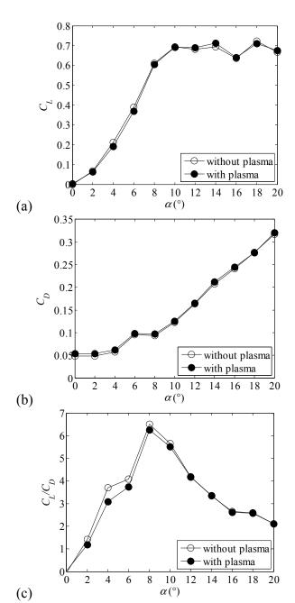
Fig. 2 Lift coefficient of the airfoil without and with plasma control of configuration 1, where two DBD plasma actuators are used. The width of each exposed electrode and the embedded electrode is 1 mm and 4 mm, respectively, and the distance of the downstream edge of the right exposed electrode to the airfoil trailing edge is 1 mm. (a) Lift coefficient; (b) drag coefficient; (c) lift-to-drag ratio.
