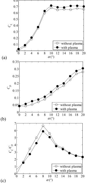
Fig. 3 Lift coefficient of the airfoil without and with plasma control of configuration 2, where two DBD plasma actuators are used. The width of each exposed electrode and the embedded electrode is 1 mm and 4 mm, respectively, and the distance of the downstream edge of the right exposed electrode to the airfoil trailing edge is zero. (a) Lift coefficient; (b) drag coefficient; (c) lift-to-drag ratio.
