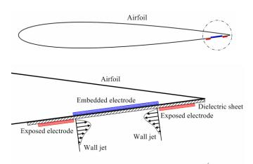
Fig. 1 DBD plasma actuators attached to the airfoil
