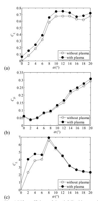
Fig. 4 Lift coefficient of the airfoil without and with plasma control of configuration 3, where one DBD plasma actuator is used. The width of the exposed electrode and the embedded electrode is 1 mm and 4 mm, respectively, and the distance of the downstream edge of the exposed electrode to the airfoil trailing edge is zero. (a) Lift coefficient; (b) drag coefficient; (c) lift-to-drag ratio.
