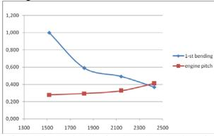
Fig. 10. First modes damping dependency on dynamic pressure
