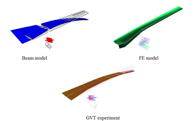
Fig. 3. Comparison of second eigenmode
