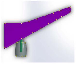
Fig. 5. Accelerometers layout
