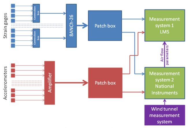
Fig. 6. Measurement systems scheme
