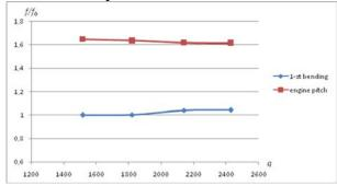
Fig. 9. First modes frequencies dependency on dynamic pressure
